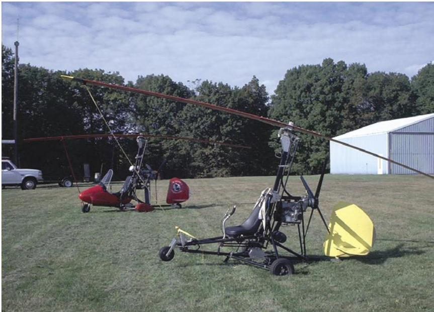
**These two Air Command Commander gyros represent the original high thrust-line design that was popular until recent advances introduced the center thrust-line design. Adding a large horizontal stabilizer to a high thrust-line gyro makes it safer to fly by reducing the tendency of the aircraft to go into a pilot induced oscillation (PIO).**
